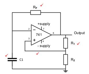
3.5.2 The output voltage of a 741 op amp astable multivibrator circuit constantly changes between + Vcc and -Vcc ✓ whereas the output of a 555 IC astable multivibrator circuit changes between +Vcc and 0 V. ✓
