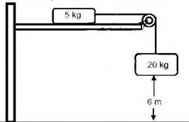
When the stationary 5 kg mass is released, the two masses begin to move. The coefficient of kinetic friction,  $\mu_k$ , between the 5 kg mass and the horizontal surface is 0,4. Ignore the effects of air friction.
