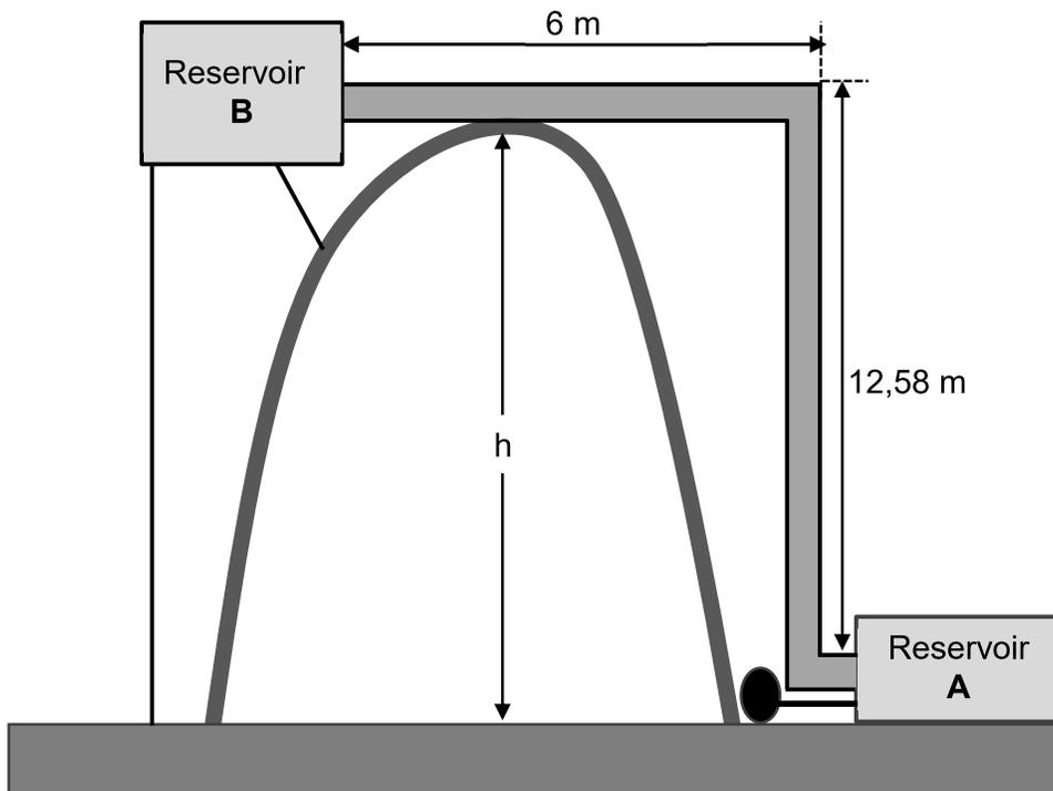
4.1 The electric water pump generates a power output of 7 200 W to pump 850 kg of water from reservoir **A** to reservoir **B** through the pipe at CONSTANT VELOCITY. Ignore the effects of friction.
