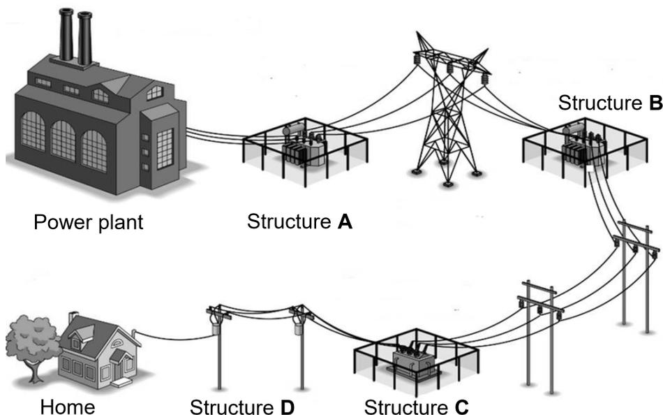
The power plant generates a voltage of 4 875 V. The transformer in structure **A** steps up the voltage that is generated by the power plant before it enters the transmission lines.
