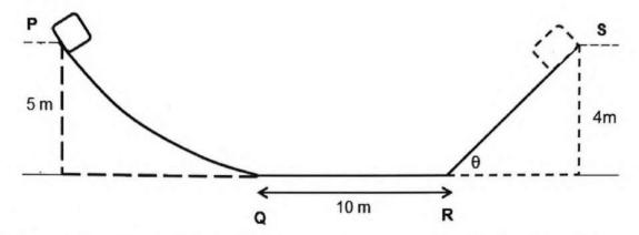
The curved section, **PQ**, is frictionless. The horizontal section, **QR**, is 10 m long and is also frictionless. Section, **RS**, is inclined at an unknown angle ( $\theta$ ) to the horizontal and is rough. The frictional force, <u>a non-conservative force</u>, between the surface and the object is 20 N.
