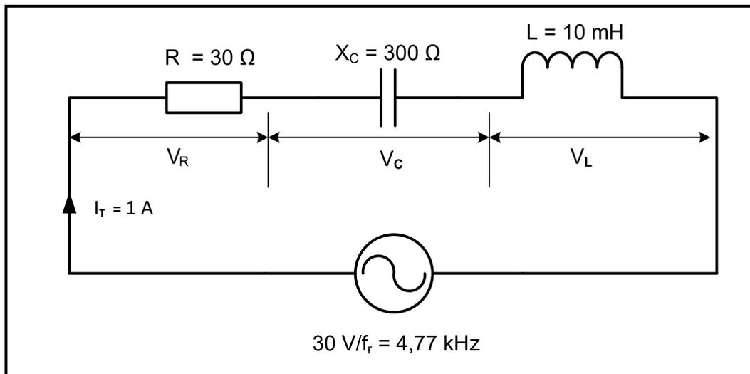
**FIGUUR 3.5: RESONANTE RLC-SERIEKRING**
