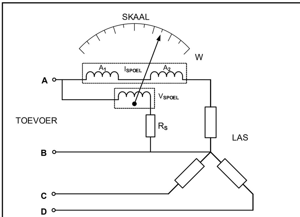
**FIGUUR 4.5: ANALOOG-WATTMETER**
