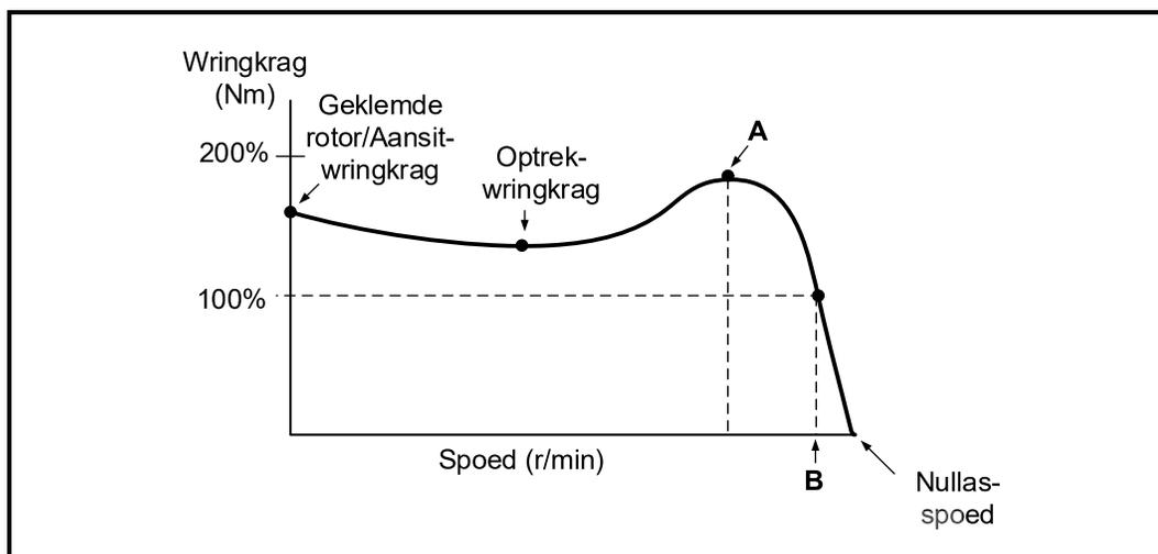
**FIGUUR 6.4: SPOED VS. WRINGKRAGKROMME**
