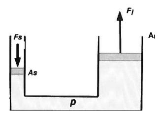
Calculate the force **F**<sub>I</sub> due to pressure exerted by force **Fs**. (3) [13]
